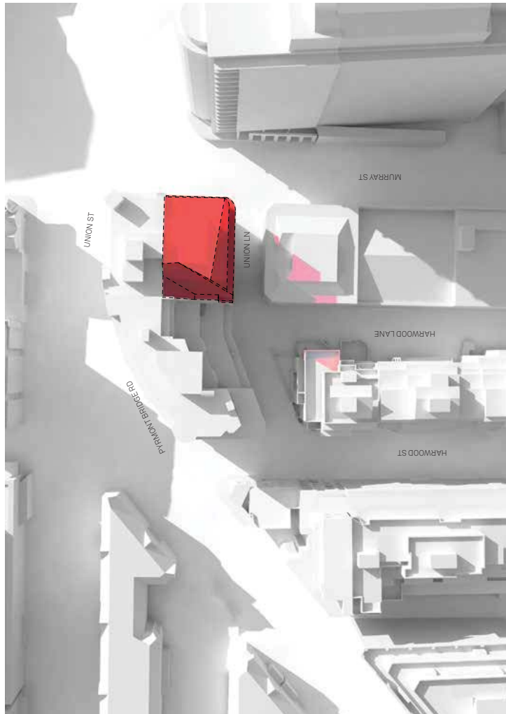
Shadow Diagram - 22nd June 9am Red shadow indicates additional overshadowing cast by proposed maximum building envelope.
