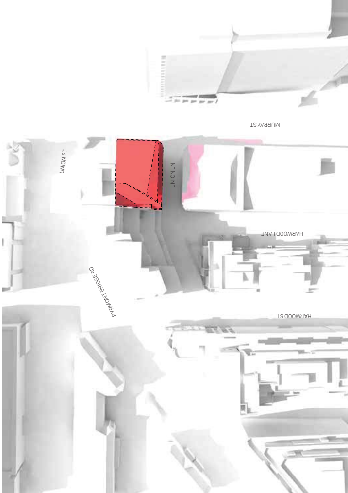
Shadow Diagram - 22nd June Noon Red shadow indicates additional overshadowing cast by proposed maximum building envelope.
