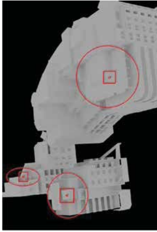
Figure 4: Rendered arbitrary areas of reduced accuracy and modified level of detail due to restrictions with the aerial LIDAR data coverage.
